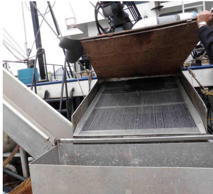
Figure 4. A De-watering box on another vessel, from the front
