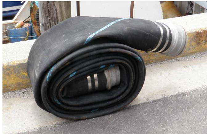
Figure 2. Example of tubing used for pumping fish
