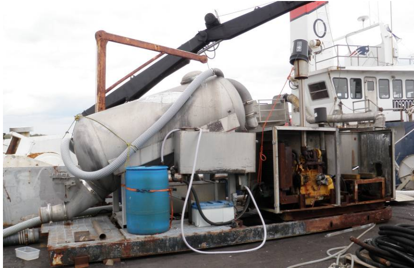
Figure 10. This pump, situated on a dock, is used to move the herring from the boat and into the dewatering box and eventually a truck or container, situated portside.
